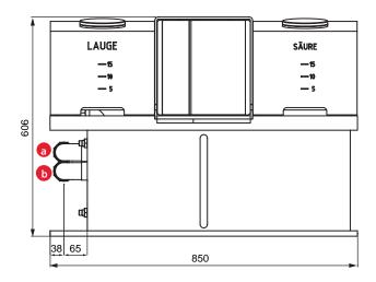
a. Water feed G 1 1/2" b. Water overflow G 1 1/2"
